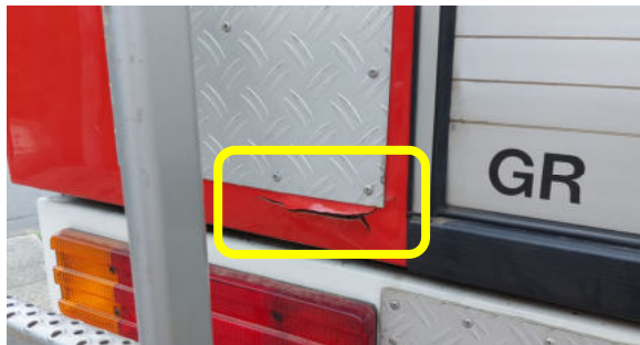
① Lack-/Rostschaden Heck links
